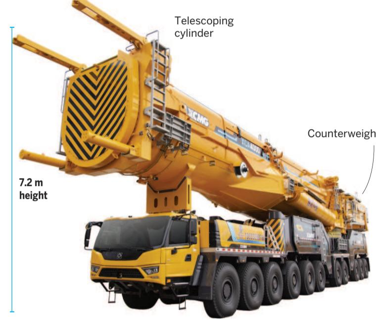
**A**t a 200-megawatt wind farm in Hengshui, Hebei province, the world's largest tonnage wheeled crane XCA4000 completed its first lift in March, lifting a 130-metric-ton nacelle, a 40-ton hub and three 95-meter-long blades weighing 28 tons each, to a height of 162 meters for assembly on the tower.
